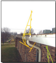
Stanchion rigged for overhang roof or gutter.
