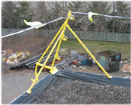
Cables moves freely around corners with clip-on rollers.
